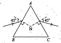
In the above diagram, what is the refractive index of material of the prism with respect to air, when the angle of deviation is 30°?
