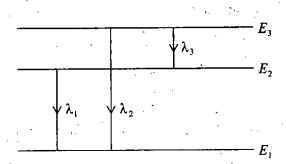
An atom has energy levels as shown in the above figure and  $E_1 < E_2 < E_3$ . The wavelengths of corresponding transitions are also shown. The relation among the wavelengths is
