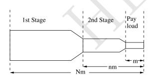
The mass of the second-stage rocket plus the payload, after first-stage burnout and separation, is nm. In each stage the ratio of container mass to initial mass (container plus fuel) is r, and the exhaust speed is V, constant relative to the engine. Note that at the end of each state when the fuel is completely exhausted, the container drops off immediately without affecting the velocity of rocket. Ignore gravity.
